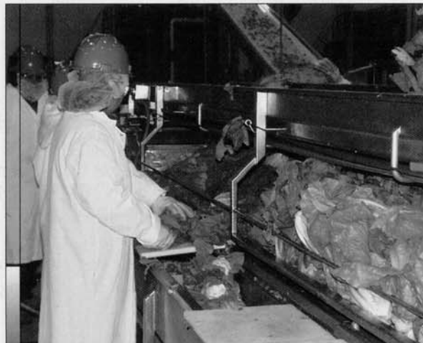
Coring is the most labor-intensive step.
