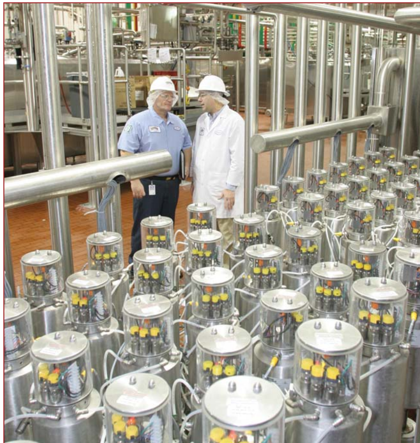
A sea of control tops on mix-proof valves attests to the serious approach to fail-safe programming to ensure allergens are removed in CIP cycles between production runs in Bakersfield. Photo by Alexander Horvath.
