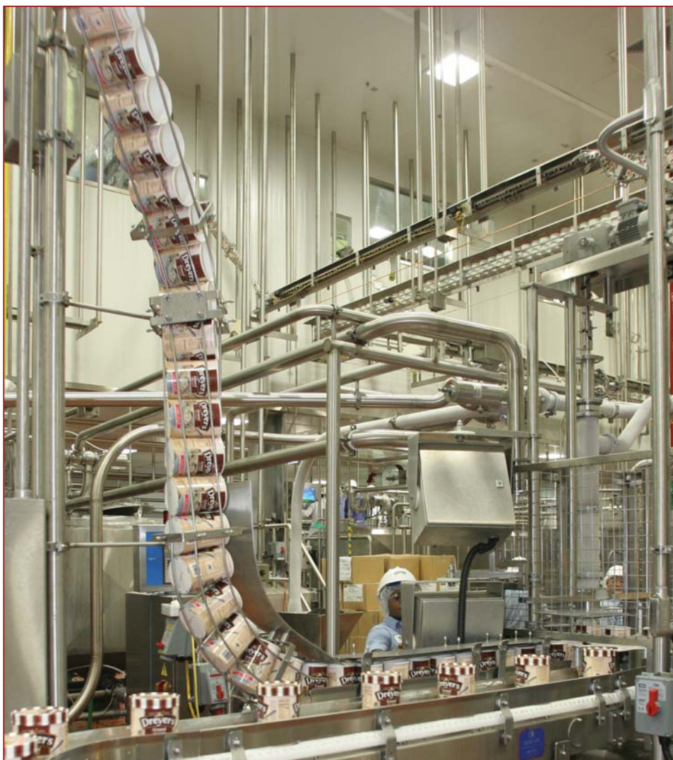
Formed cartons feed down a wire-guided conveyor to a filling machine in the new production area at Dreyer’s Grand Ice Cream’s Bakersfield, CA, plant. Photo by Alexander Horvath.
