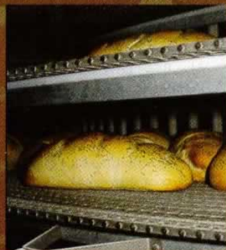
Par-baked loaves must cool thoroughly before packaging to stabilize their structure and crust.
